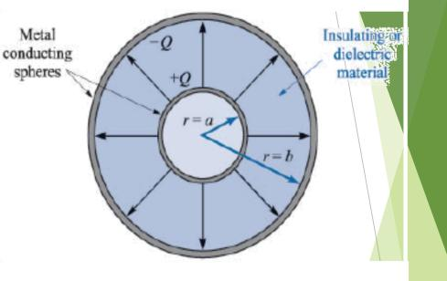
The electric flux in the region between a pair of charged concentric spheres. The direction and magnitude of D are not functions of the dielectric between the spheres
